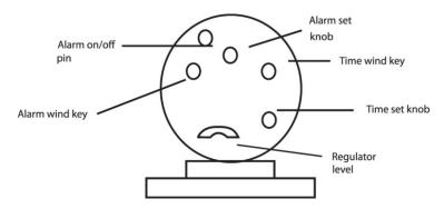
**To Set the Time:** Turn the time set knob to the correct time. Wind the time key fully in the direction the arrow indicates.
