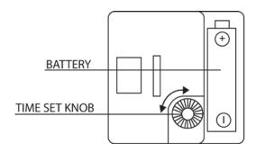
**Battery:** Insert one new AA Alkaline battery according to the polarity marked in the battery compartment.
