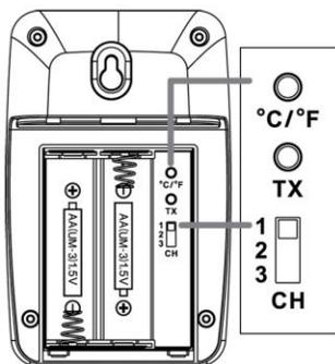
1. Slide the battery cover down, then lift off the back of the transmitter.
