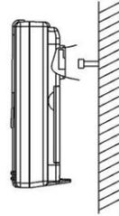
**Note:** Always ensure that the transmitter locks onto the screw before releasing.
