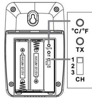
Press and release the CH button to view channel 1, 2 or 3 on the Weather Station when multiple transmitters are used.
