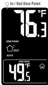
Dew point is the saturation point of the air, or the temperature to which the air has to be cooled in order to create condensation. The higher the dew points, the higher the moisture content of the air at a given temperature. Dew Point Temperature is the absolute measure of the moisture in the air at a given temperature. Relative humidity is the relative measure of moisture in the air at a certain temperature.
