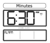
**Deactivate | Activate:** The alarm is active when set. Press and release the ALARM button to deactivate or activate the alarm.
