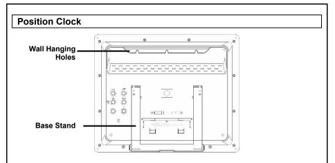
When positioning the atomic digital clock it is always best to have the front or the back facing Ft. Collins, Colorado for best WWVB signal reception.
