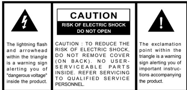
The lightning flash and arrowhead within the triangle is a warning sign alerting you of "dangerous voltage" inside the product.
