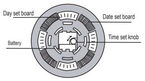
Battery:Insert one new AA Alkaline battery according to the
