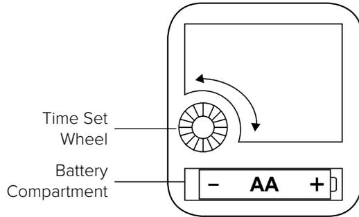
**Note:** The quartz movement will keep the clock running accurately. If the clock does not operate, or steadily loses time, replace the battery.
