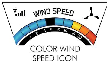
The wind cup icon will spin at varying speeds according to the current speed.
